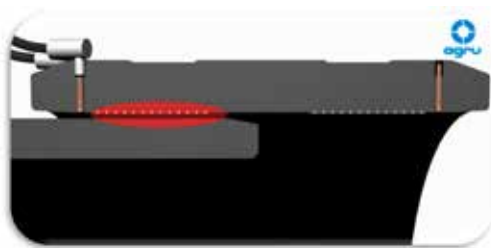
Figure C.12: Principle of the bifilar welding
